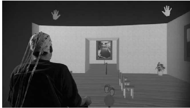
Fig. 3 Exploring a virtual museum using a BCI and high-level commands [46].
