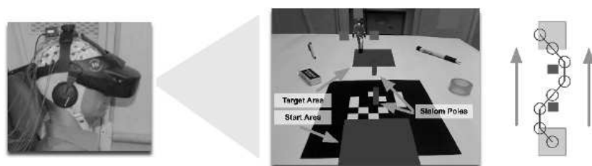
Fig. 7 The middle picture shows a screenshot of how the user saw the scene through the HMD seen in the left picture. The 3D graphics were tracked to the underlying fiducial marker. The participants were instructed to navigate the avatar through the slalom like in the picture on the right [18, 19].
