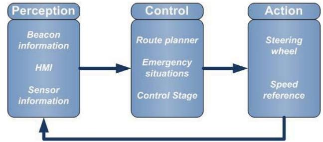
Figure 8. Control Scheme of the Cyber car.
