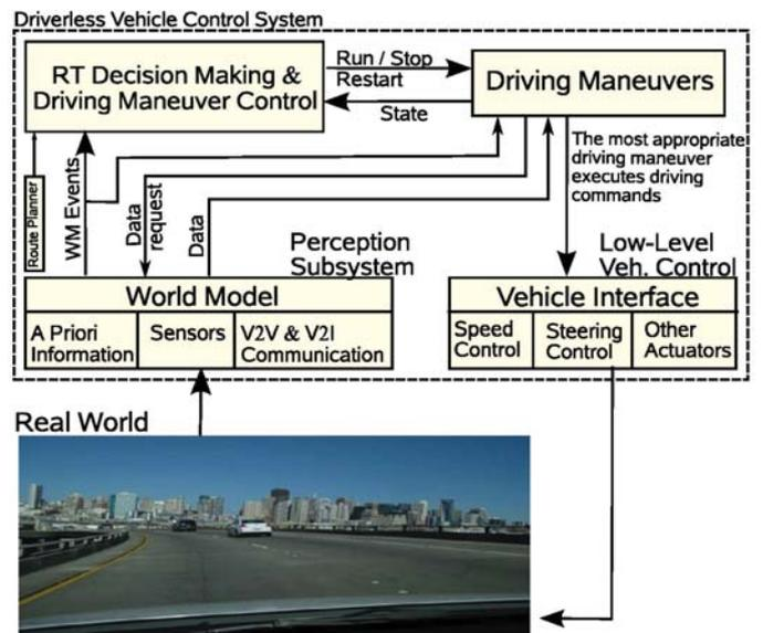
Figure 4. Driverless Vehicle Decision and Control System [25]
