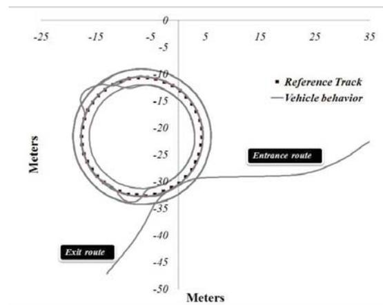
Figure 10. Cybercar's behavior on the roundabout, lane change maneuver taking the first exit.
