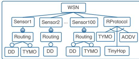
Figure 2: Network Configuration with Energy Efficient Protocols
