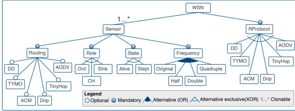
Figure 1: Feature Model for the ITS Scenario
