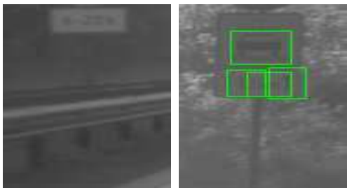
Fig. 6. Some bad results obtained with the region-growing method due to no seed selection (left) or a low contrast (right).
