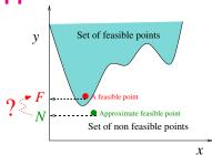
N, optimal solution of R, not a feasible point of P but (may be) a good starting point:
