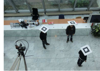
Fig. 6. Subjects wearing hats with markers and camera with wide angle lens at INRIA's hall
