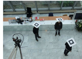
Fig. 6. Subjects wearing hats with markers and camera with wide angle lens at INRIA's hall
