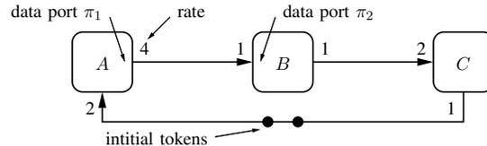
Fig. 1 shows a simple SDF graph with three interconnected actors *A*, *B* and *C*. Actor *A* has one input and one output port, whose rates are 2 and 4, respectively.
