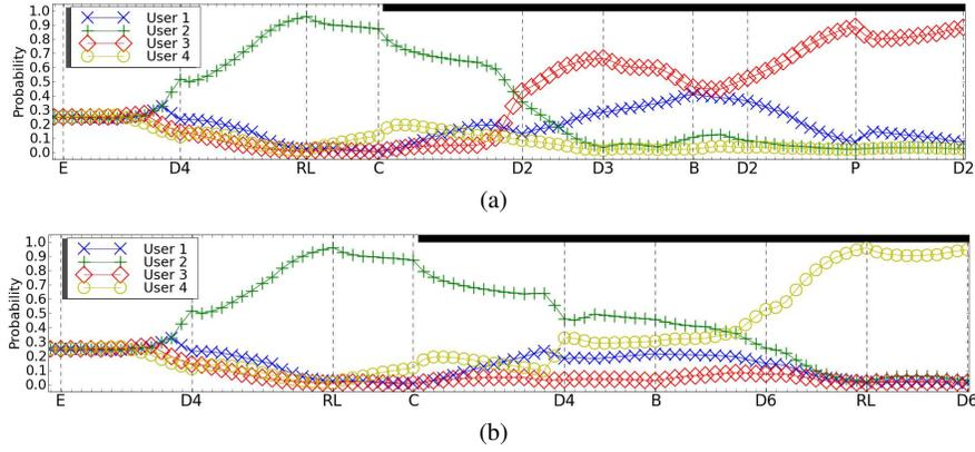
**Fig. 6** Scenarios where (a) user 3 and (b) user 4 take the robot from user 2 in the cafeteria. The user probability is displayed. The dotted lines indicate the steps where a user stops at a goal. The black region indicates when a new user is steering the robot.
