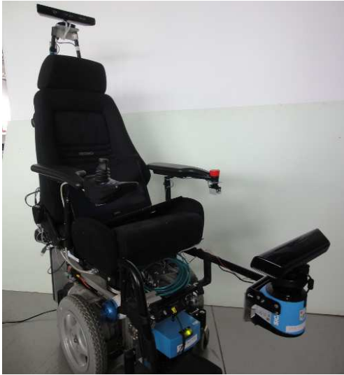
Fig. 4. Robotic wheelchair used for the described experiments. The mobile base includes all the electronic components and the computer in charge of the low level control of the wheelchair
