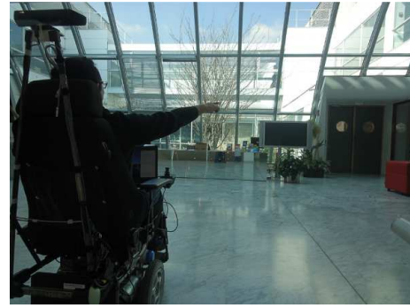
Fig. 7. A user pointing to his desired destination. The idea is to be able to understand which are the most probable goal given the direction of the gesture
