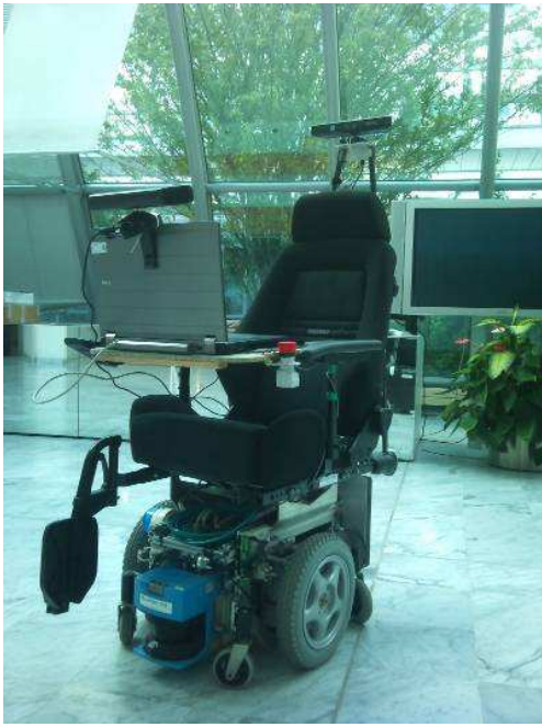
Fig. 5. Robotic wheelchair used for the described experiments. The mobile base includes all the electronic components and the computer in charge of the low level control of the wheelchair
