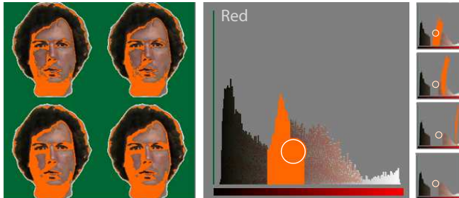
Figure 5: Applying the paintbrush on a view temporarily freezes all histograms (middle). At mouse release, painted pixels jump to their new location (right).
