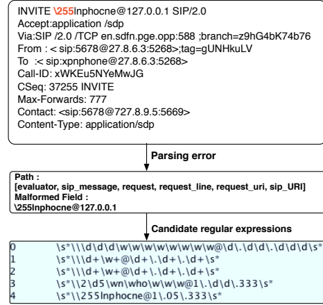
Fig. 2. Example of a malformed SIP message and the set of candidate regular expressions.
