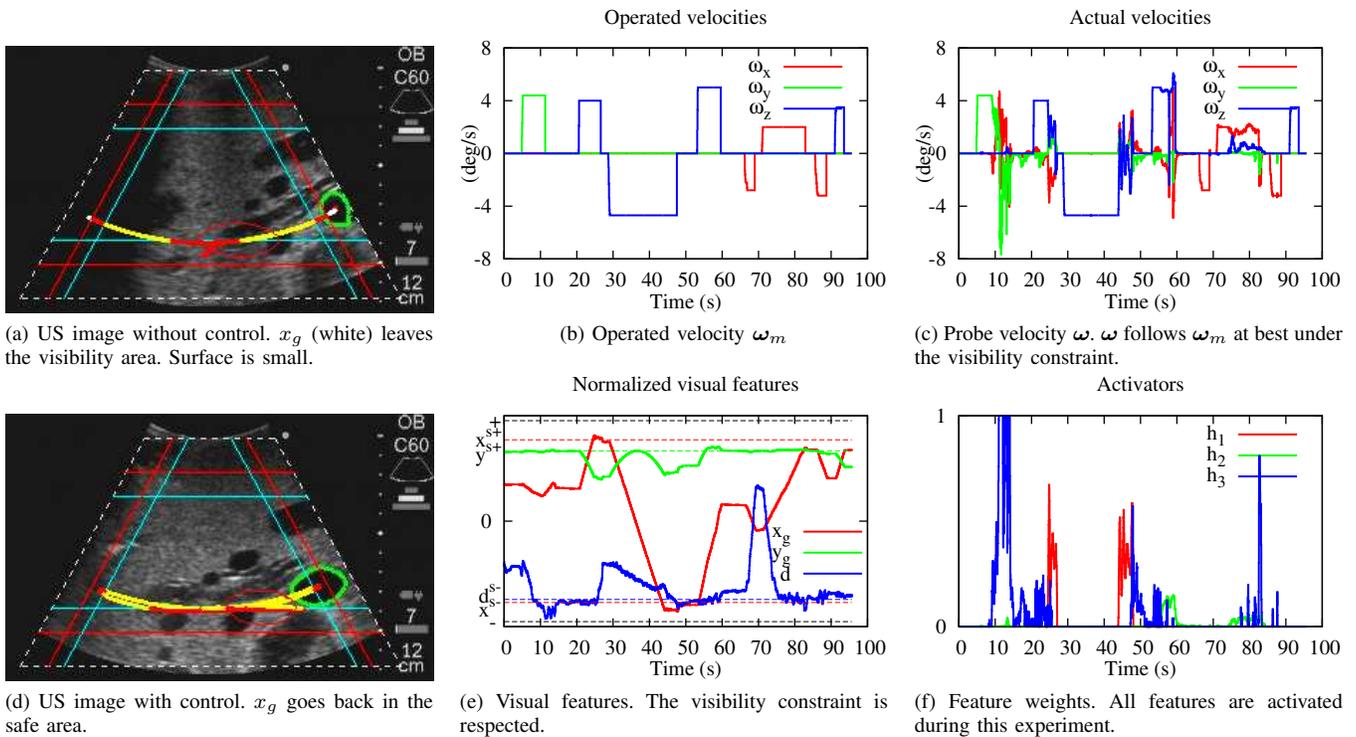
Fig. 7. Results on the real phantom. US image without (a) and with (d) the control law. Operated velocity  $\omega_m$  (b) and actual probe velocity  $\omega$  (c). Normalized visual features (e) and corresponding weights (f).
