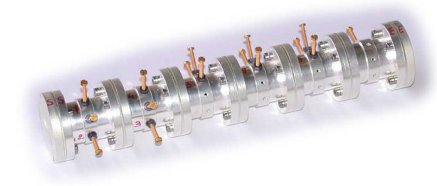
Fig. 1. A microwave filter.
