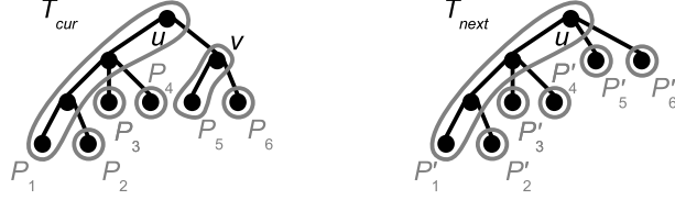
Fig. 5. Left: a tree T_{cur} with its path partition \mathcal{P}_{cur} = \{P_1, P_2, P_3, P_4, P_5, P_6\} whose partition tree T_p^{cur} has height 2. Right: the tree T_{next} resulting from the contraction of edge uv in T_{cur} , together with its path partition \mathcal{P}_{next} = \{P'_1, P'_2, P'_3, P'_4, P'_5, P'_6\} . All the paths in \mathcal{P}_{next} are the same as those in \mathcal{P}_{cur} , except P'_5 which has lost node v . The height of T_p^{next} decreased, it is now 1.
