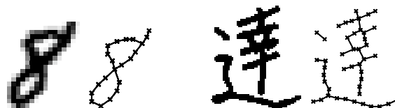
Figure 1.14: For digits and Chinese characters: (left) original characters, (right) thinned and subsampled characters.
