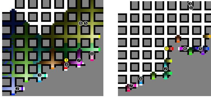
Fig. 3. Resulting potential values from the wavefront propagation algorithm when stopped on the robot computing its assigned frontier (left) and using the parallel wavefront computation (right). Robot computing its allocation is in yellow. Cell color is white when no potential value has been computed in this cell, otherwise it has the color of the frontier associated with minimum potential values computed in that cell.
