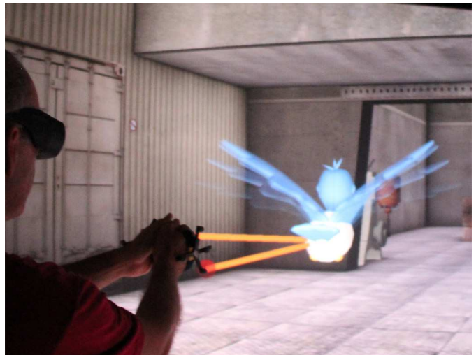
Fig. 1. One of the novel locomotion techniques we propose: the Virtual Companion is implemented with a bird which both warns the user about physical workspace limits and allows navigation in the environment using a metaphor with virtual reins.
