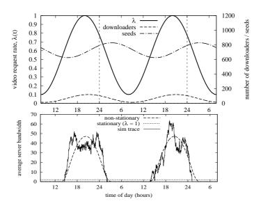
Figure 8: Temporal evolution of video request rate (top plot, left y axes) number of downloaders/seeds (top plot, right y axes), and average server bandwidth  $\overline{S}(t)$  (bottom plot), in the *set-top-box* system.
