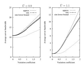
Figure 4: Comparison of average server bandwidth with  $\overline{N} = 100$ ,  $d = d_v$ ,  $\overline{T} = T_v$ , as function of the variation coefficient of peer upload bandwidth, for  $\overline{U} = 0.9$  (left plot) and for  $\overline{U} = 1.1$  (right plot).
