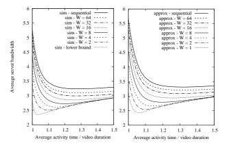
Figure 6: Average server bandwidth as function of the ratio  $\overline{T}/T_v$  between average activity time and video duration, keeping fixed  $\overline{N}=100,\,d=d_v,\,\gamma=1$ , for different values of the number of segments W. Comparison between simulation (left plot) and approximate analysis (right plot).
