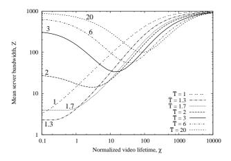
Figure 10: Average server bandwidth Z as function of the normalized video lifetime  $\chi$ , for different values of user activity period  $\overline{T}$ , in the case of  $\Lambda = 1000$ .
