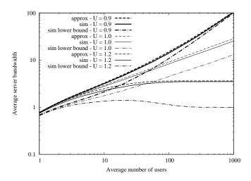
Figure 1: Comparison of average server bandwidth in the case  $d = d_v$ , as function of the average number of users  $\overline{N}$ , for different values of  $\overline{U}$ , in the absence of seeds.
