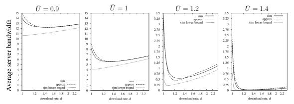
Figure 3: Average server bandwidth as function of the target download rate d, for different values of  $\overline{U}$ , with  $\overline{N} = 100$ ,  $\overline{T} = T_v$ .
