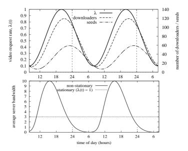
Figure 7: Temporal evolution of video request rate (top plot, left y axes), number of downloaders/seeds (top plot, right y axes), and average server bandwidth  $\overline{S}(t)$  (bottom plot), in the *software-based* system.
