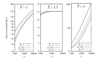
Figure 11: Average server bandwidth Z as function of  $\Lambda$ , for different values of the Zipf's exponent  $\alpha$ , and fixed  $\chi=10$ . The user activity period is either  $\overline{T}=1$  (left plot), or  $\overline{T}=1.5$  (middle plot) or  $\overline{T}=3$  (right plot).
