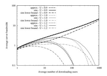
Figure 2: Comparison of average server bandwidth in the case  $d=d_v$ , as function of the number of downloading users  $\overline{N}_d$ , for different values of  $\overline{U}$ , in the presence of  $\overline{N}_{seed}=0.1\cdot\overline{N}_d$  seeds.
