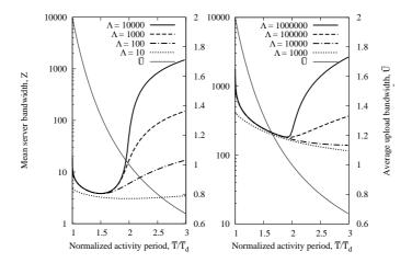
Figure 9: Average server bandwidth Z as function of normalized user activity period  $\overline{T}/\overline{T}_d$ , for  $\chi=1$  (left plot) and  $\chi=100$  (right plot), and different values of  $\Lambda$ . The associated average upload bandwidth  $\overline{U}=2/\overline{T}$  is reported on the right y axes.
