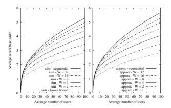
Figure 5: Average server bandwidth as function of the number of users, with  $\overline{T} = T_v$ ,  $d = d_v$ ,  $\gamma = 1$ , for different values of the number of segments W. Comparison between simulation (left plot) and approximate analysis (right plot).
