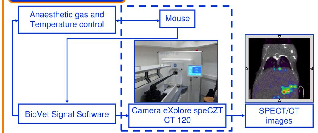
Diagram: The pressure sensor (balloon) is set up under the abdomen of mice. Mice are breathing freely air with anaesthetic gas (Isoflurane). The camera eXplore speCZT CT 120 is a coupling SPECT and CT images. The picture above present liver metastasis from PROb-mNIS adenocarcinoma injected in NOD-SCID mouse.
