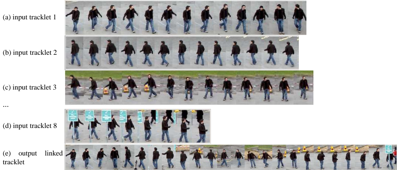
Figure 6: Linking algorithm inputs and output. The length of the output tracklet is the sum of the lengths of the inputs tracklets. In this example, the input tracklets length is between 8 and 120 frames and the output length is 348 frames.
