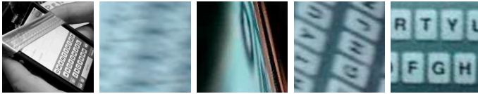
(a) Occlusion (b) Camera + device movements. (c) Device movements only. Figure 5: Permanent occlusions (a) and quick camera movements (c) are tolerated with errors. However, when both camera and device shake excessively (b) the high blur level prevents the detection of the screen.
