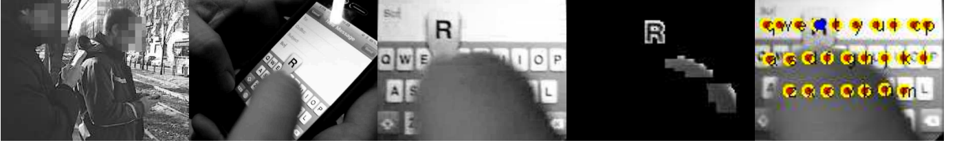
(a) Envisioned attack settings. (b) Input of Phase 1. (c) Input of Phase 2. (d) Input of Phase 3. (e) Output (i.e., the 'R' key).
