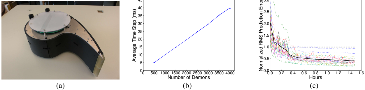
Figure 2: A robot learning many pieces of knowledge. (a) The robot. (b) The time requirement scales linearly with the available computation, with timescales that are reasonable for robots. (c) Learning many predictions in parallel about different policies with substantial reductions in error in 30 minutes, and improving with additional experience. The prediction error is the measured difference between predictions and empirical returns on a separate evaluation run. For each question, the root-mean-square error is normalized by the sample standard deviation over the evaluation set. Thus, normalized errors below 1 indicate the portion of the variance in the empirical returns that the robot is able to predict.
