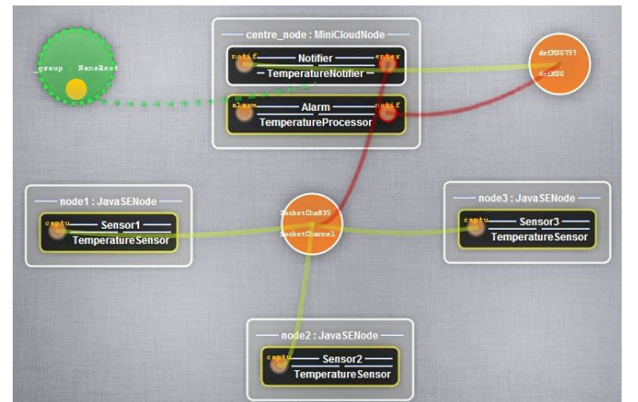
Figure 2: Architecture of the system using the Kevoree graphical notation
