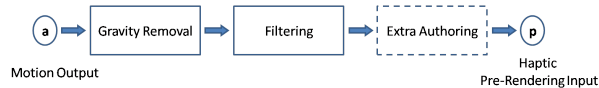
Figure 3: Processing Overview. The gravity is removed from the accelerations motion signals captured. Optionally extra processing can be performed such as low-pass filtering.
