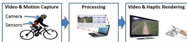
Figure 1: Workflow Overview. Data are simultaneously captured by a camera and a motion sensor. Then motion data are converted into a signal suitable for the dedicated haptic renderer. Finally both video and motion are rendered simultaneously.
