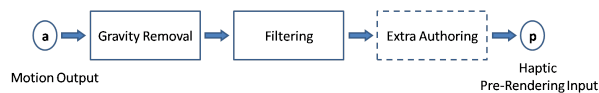
Figure 3: Processing Overview. The gravity is removed from the accelerations motion signals captured. Optionally extra processing can be performed such as low-pass filtering.
