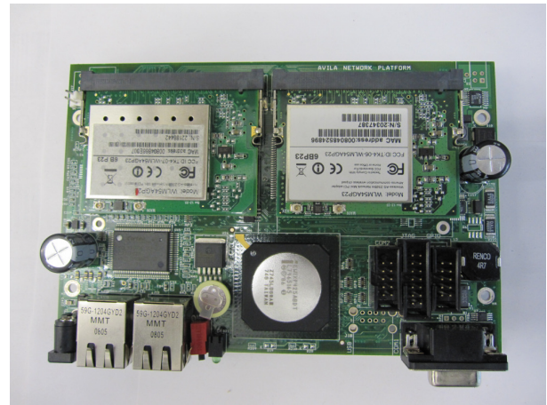
Fig. 1. Gateworks Avila multi-radio platform equipped with two Compex WLMAG54-23dBm mini PCI cards.
