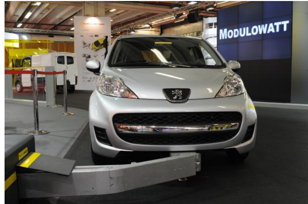
Fig. 1. Demonstration of the docking station for recharging during the Paris Motor Show 2010.
