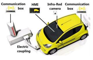
Fig. 2. System architecture
