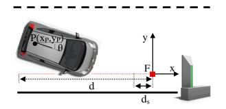
Fig. 3. Geometry of the docking maneuver.
