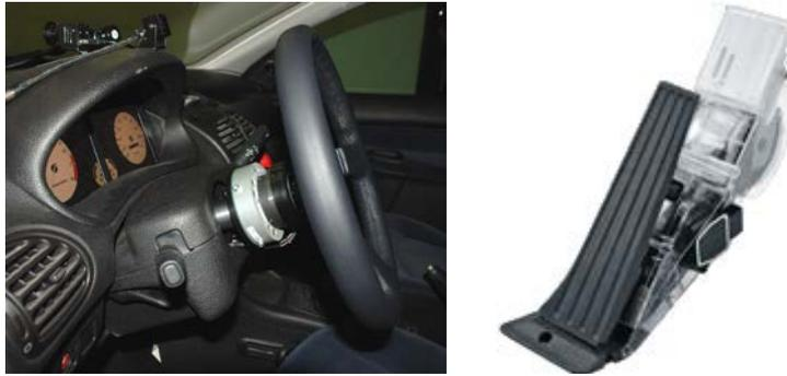
Figure 6 By wire Steering wheel and active pedal
