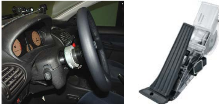
Figure 6 By wire Steering wheel and active pedal
