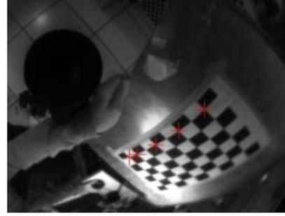
Fig. 6. Estimation of the focal from line image points
