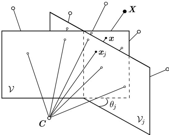
**Fig. 2** A camera samples the bundle of rays that pass through the optical centre  $C$ . Two different views, separated by a rotation of  $\theta_j$ , are indicated by the planes  $\mathcal{V}$  and  $\mathcal{V}_j$ . Corresponding points  $x$  and  $x_j$ , which are images of  $X$ , are related by a projective transformation  $H$  of the projective space  $P^2$ .
