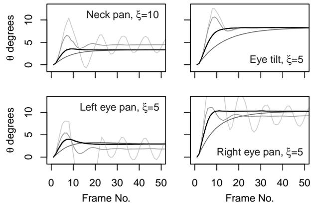
**Fig. 10** Response of the active binocular head motors to a step input. A static face was detected and the cameras rotated to fixate on the face. The damping factor was tuned so as to give a fast rise-time with minimal overshoot.
