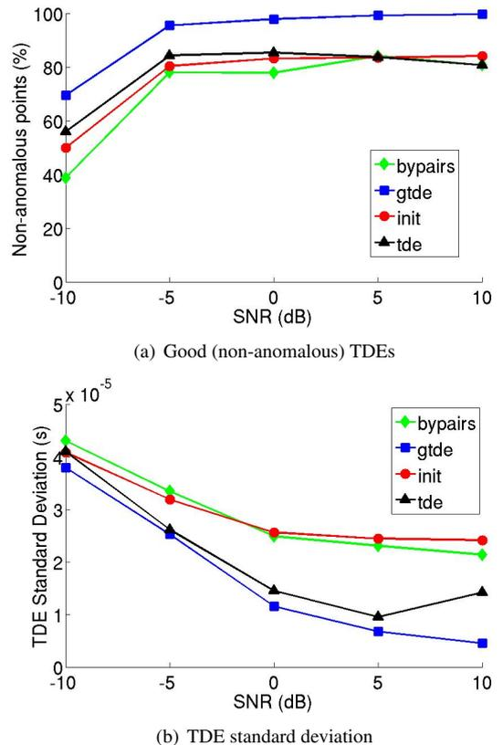
**Fig. 1.** (Best seen in color) TDE method comparison based on random speech fragments. The plots show (a) the percentage of good TDEs and (c) the standard deviation as a function of SNR in an anechoic setup ( $T_{60} = 0$ ).
