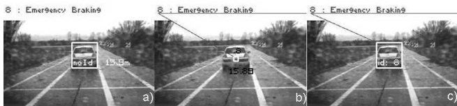
Fig. 11. Telecom enriched detection: a) a car is detected thanks to the lidar and a message is received from vehicle 8. b) an object identified as 8 is perceived and localized in the scene. c) both detections are associated: the car in front is sending an emergency brake message.
