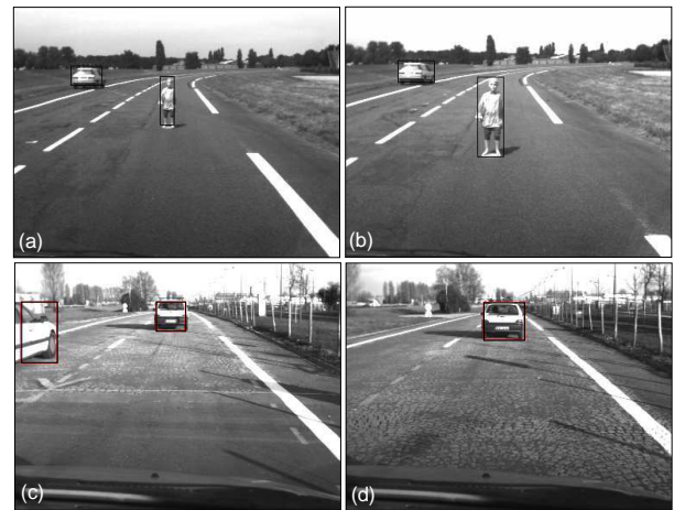
Fig. 11. Examples of bounding boxes around multiple objects: (a)(b) a car and a pedestrian; (c)(d) two cars on a paved road, which is a typical periodic noisy texture.
