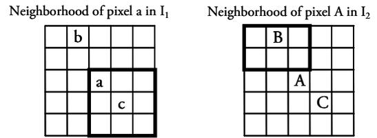
Fig. 5. Definition of neighborhood  $N(a, A)$  of pixel match  $(a, A)$ . It is a set of matches included in the two  $5 \times 5$ -neighborhood  $N_5(a)$  and  $N_5(A)$  of pixels  $a$  and  $A$ . Possible matches for  $b$  (resp.  $C$ ) are in the  $3 \times 3$  black frame centered at  $B$  (resp.  $c$ ).
