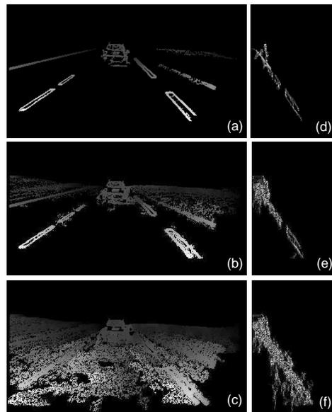
Fig. 7. Results of the quasi-dense matching algorithm on our test images for different values of  $t$ : (a)  $t = 0.05$ , (b)  $t = 0.02$ , (c)  $t = 0.01$ . (d)(e)(f) corresponding "v-disparity" images. When the threshold  $t$  is lowered, numerous correlated errors appear and straight lines in the "v-disparity" image get thicker.
