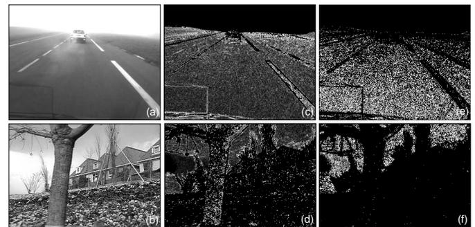
Fig. 6. Comparison of roughness of (a) our road image under foggy weather; (b) image used by Lhuillier; (c)(d) white pixels  $x$  where  $0 < s(x) < 0.05$ ; (e)(f) white pixels  $x$  where  $0 < s(x) < 0.01$ .
