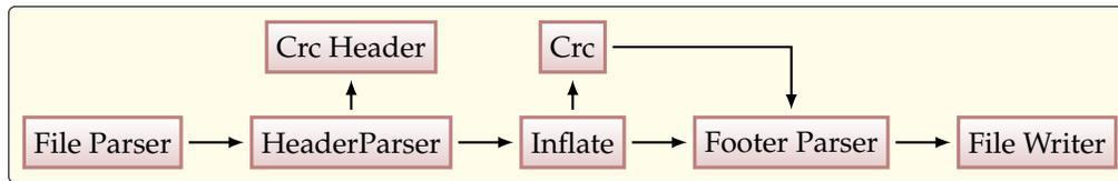
Figure 5: Top level view of RVC-CAL Gzip Decoder
