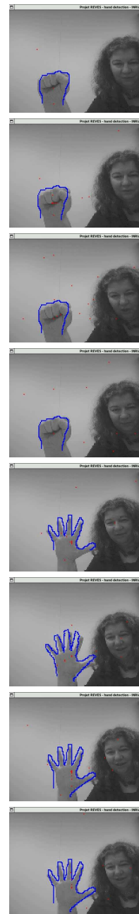
Fig. 6. Example of detection on a video sequence in natural light environment. Blue shapes show the detected model, red points correspond to the position (origin of the models) (x, y) of all individuals of the current population.
