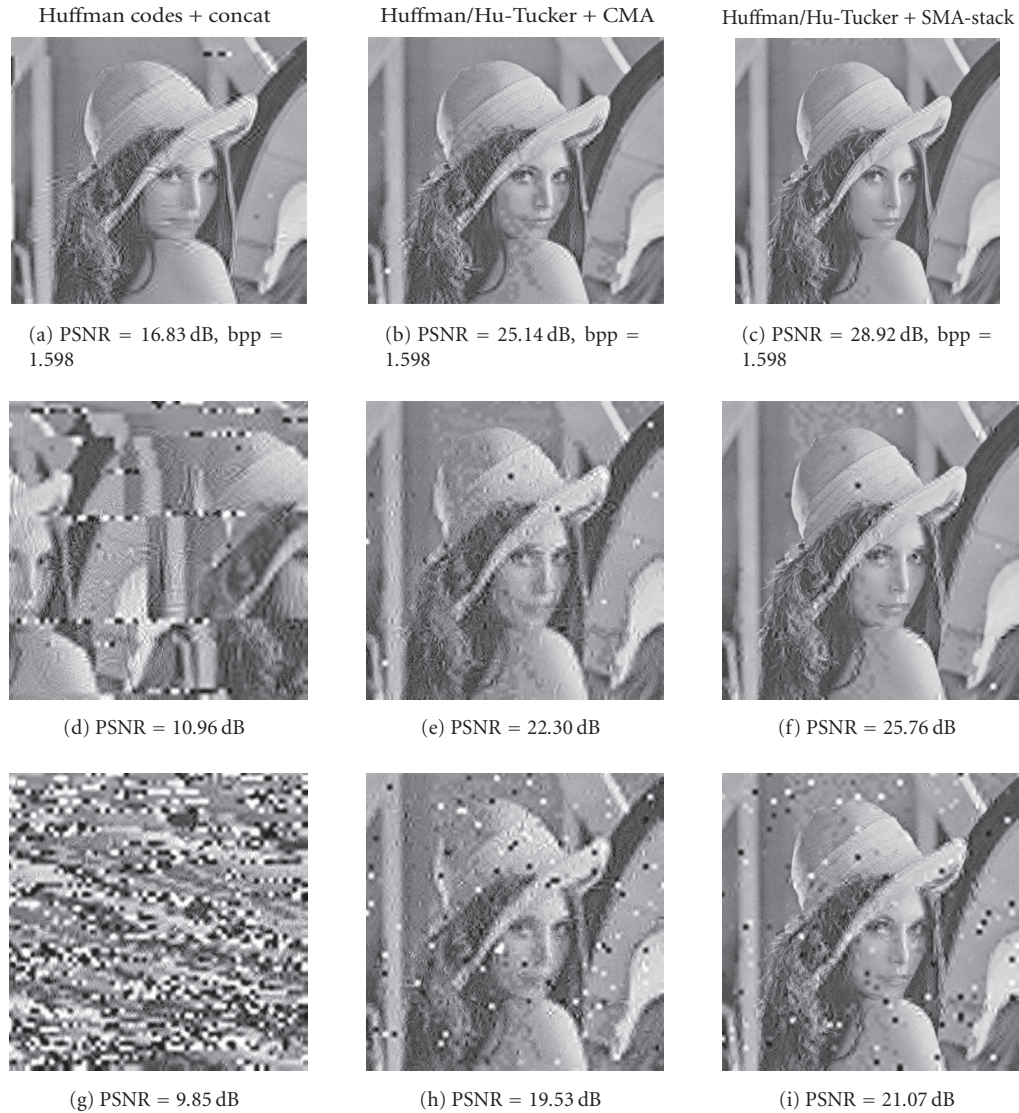
FIGURE 11: PSNR performance and visual quality obtained, respectively, with concatenated Huffman codes and two transmission schemes using Hu-Tucker codes for low subband and Huffman codes for high subbands. These schemes use, respectively, the CMA algorithm and the SMA-stack algorithm. The channel bit error rates are 0.0001 (top images), 0.001 (middle images), and 0.01 (bottom images).
