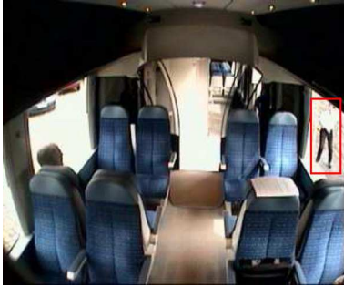
FIGURE 6: Shows a person (on the right) who is seen through a window in the wall. In this case, the repositioning algorithm has to take into account the particular situation and to avoid repositioning the person inside the train when it is outside.
