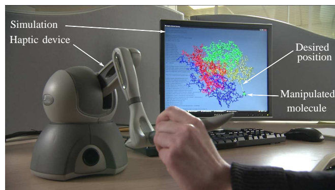
Fig. 1. Manipulation of a tetraethylammonium (TEA) around a potassium channel (KcsA). A haptic device is used to control the molecule and feel the interactions between the ligand and the protein derived thanks to the adaptive simulation
