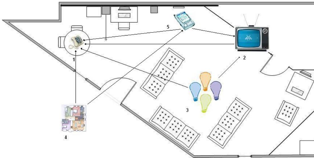
**Figure 17** When the smartphone (5) is entering in the room, it is discovered by the other devices and applications. It is a context information provider for the phone (1) and the television set (2), and it asks context information to the location service (4).
