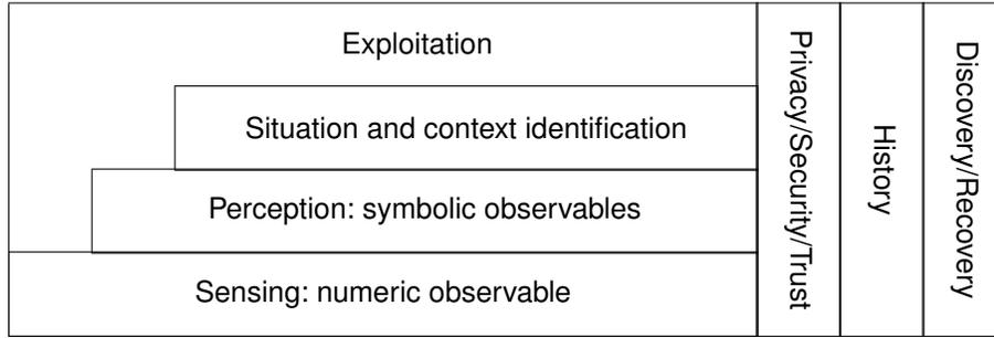
**Figure 3** Model for context management in pervasive computing. Data coming from sensors are aggregated and elaborated into the context used by applications (reproduced from [9]). We do not consider the orthogonal aspects (discovery, history and security).
