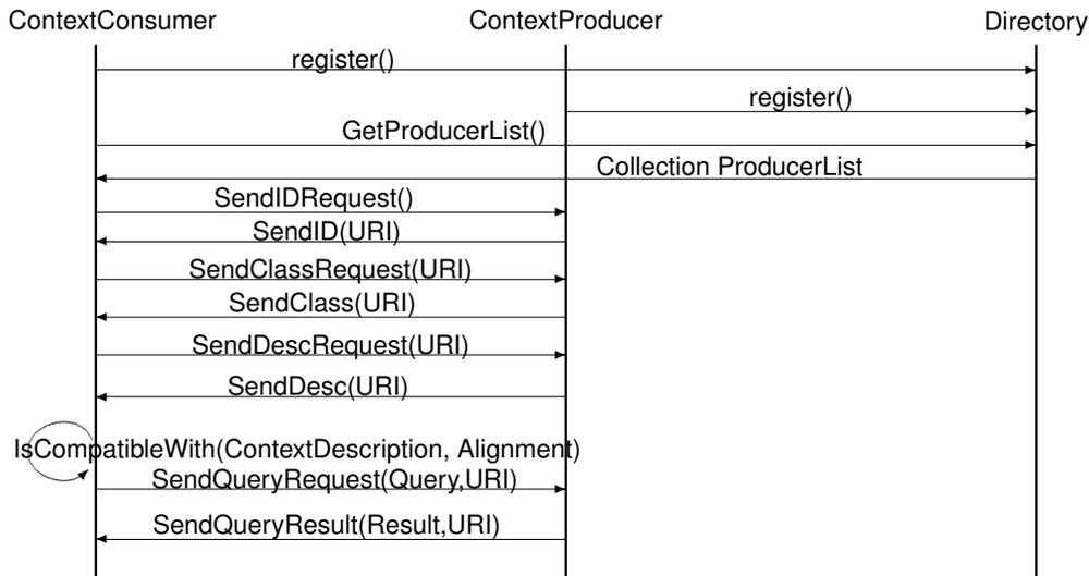
**Figure 13** The activity diagram corresponding to the protocol.
