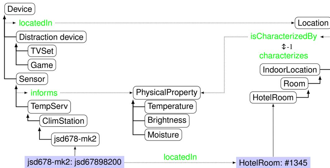
**Figure 6** Specific ontologies related to the objects found in the environment. They refine the general purpose ontologies of Figure 5 with new concepts to be considered (instances are denoted by grey rectangles and linked to their classes by thin arrows).
