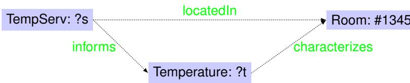
**Figure 7** A query graph pattern (question marks instead of instance names introduce free variables). It can correspond to the information that an application requires from the environment (here the temperature measured in a room). This information is expressed in function of the specific ontologies of Figure 6.
