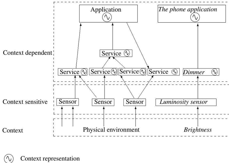
**Figure 10** A context information manager component is embedded in each device and application: any component can embed a context management library which it uses for its own purposes. It can also use this library for providing context information to other components.
