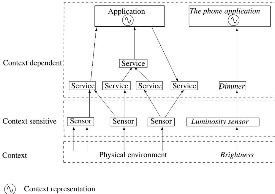
**Figure 1** General architecture of a pervasive computing environment: sensors, e.g., Luminosity sensor, provide information about the environment (here the Brightness). These are provided as services enabling other services or applications to assess the context of some task (the luminosity at some place in the physical environment). Context representation is handled in applications which need it (mentions in italics denote examples, arrows denote information flow).
