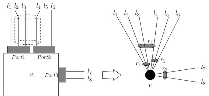
Fig. 1. Example of localized risks: link  $l_4$  shares risk  $r_2$ , corresponding to Port 2 failure, with  $l_5$  and  $l_6$ , and shares risk  $r_4$ , corresponding to a conduit cut, with links  $l_2$  and  $l_3$ .
