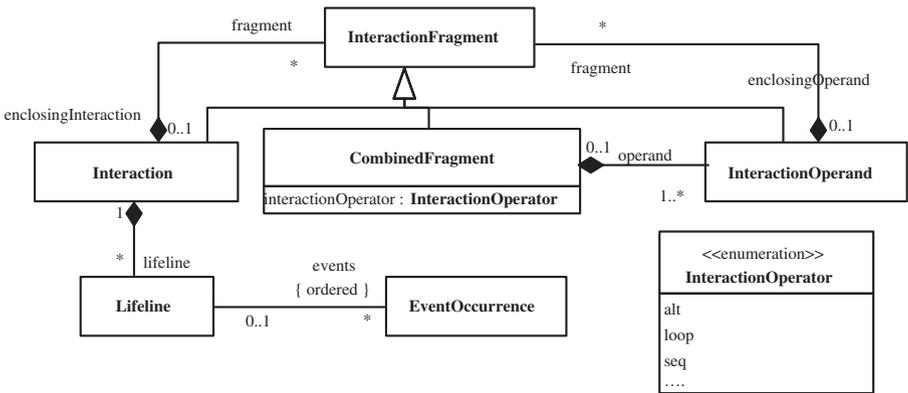
**Fig. 2.** UML 2.0 metamodel: Interaction part [5]
