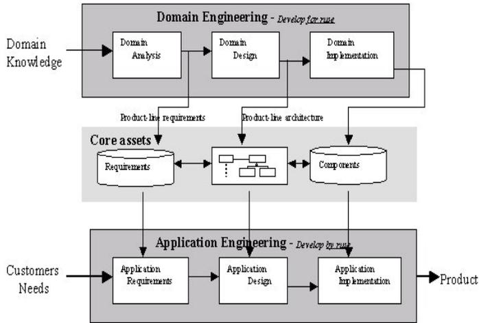
**Figure 1. The general process for Product Lines Engineering**
