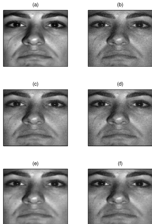
Fig. 11. Face image denoising. Top row: original face (left), noisy face (right). Denoising results using (7). Middle row: \lambda = 0.3 using the learned analysis operator (left) and the finite difference operator (right). Bottom row: same as middle row with \lambda = 0.1 .
