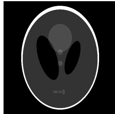
Fig. 5. A 512 by 512 Shepp-Logan phantom image which was used as the training image.
