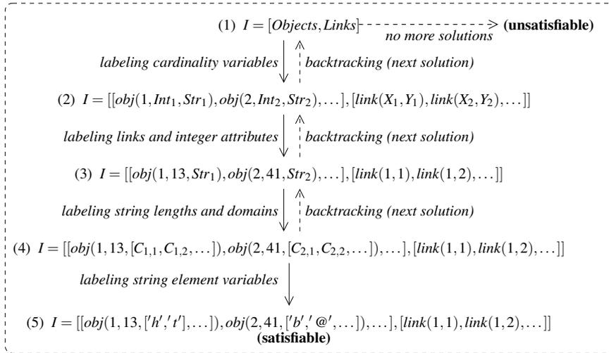
Fig. 2: EMFtoCSP’s search process, showing the different instantiation levels of the solution  $I$ : (1) cardinalities; (2) partial object diagram with potential links; (3) with ground links and numeric attributes; (4) with strings instantiated as lists; and (5) fully ground (i.e., satisfiable).
