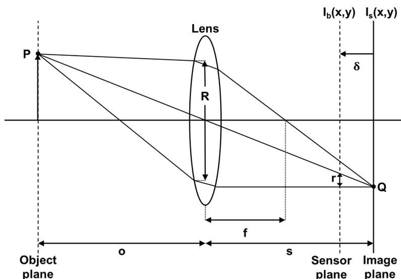
However, by using a real optical system, the object plane is not a plane but an area where the projected image will be sharp. This area corresponds to a depth of field (Figure 2) and can be calculated by the following equations:
